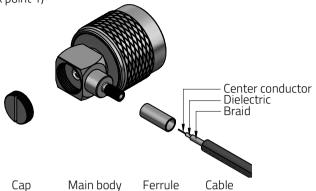
Step 2. Please slide ferrule onto cable and splay out cable braid
